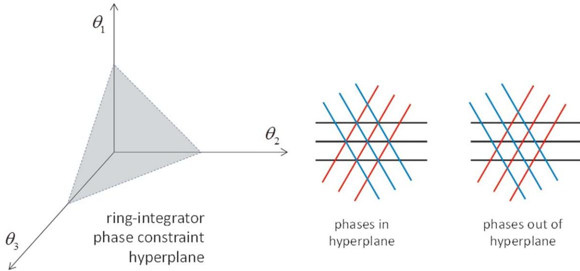
**FIGURE 3.** Phase space constraint for a 2-D example. A 2-D grid cell uses three ring-integrators configured for motion in three different directions: 0, 120, and 240°. The individual neurons of a given ring-integrator are stripe cells with different phases along the same direction. The 2-D grid cell fires when all three of its inputs (from different rings) are active. This occurs in the example on the left, “phases in hyperplane.” This requires a specific phase
