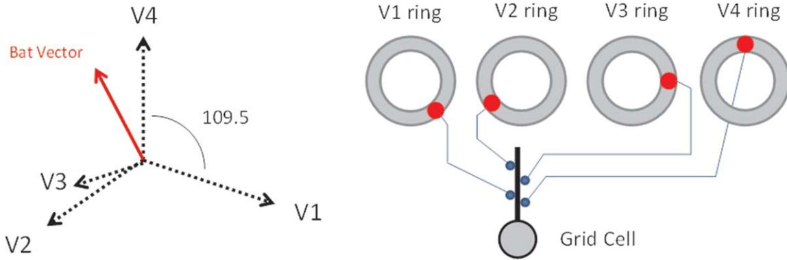
**FIGURE 2.** 3-D Grid Cell Model. Left: A three-dimensional movement vector (thick red arrow) is projected onto each of the four ring-integrator orientations. The resulting vectors are then translated into a rotational phase rate that moves the bumps around each ring. Projection vectors with “+” signs produce positive phase rotations and vectors with “-” signs produce negative phase rotations. Note that these vectors are defined in the world
