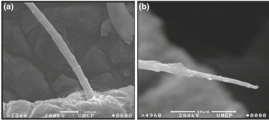
**Fig. 8.2** Scanning electron microscope images of hairs from the wing membrane of the Big Brown Bat, *Eptesicus fuscus*. **a** Base of a hair (diameter  $\sim 5 \mu\text{m}$ ) protruding from a dome-like structure. Note the coronal scale pattern. **b** Tip of a hair (diameter  $\sim 400 \text{nm}$ ). The calibration bars located on the bottom of both images indicate  $10 \mu\text{m}$
