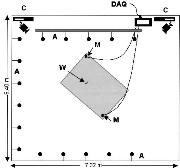
FIG. 2. Plan view of flight room and array layout. **A**: Microphone array; **M**: Ultrasound advice microphones; **C**: High-speed digital video cameras running at 240 frames per second; **DAQ**: Data acquisition systems; IoTech WaveBook, 2 channels at 250 kHz each and National Instruments AT-MIO-16-E-1 board, 16 channels at 20 kHz each; **W**: Tethered worm. Shaded area represents the calibrated space (within which the path of the bat may be accurately reconstructed from the camera views).
