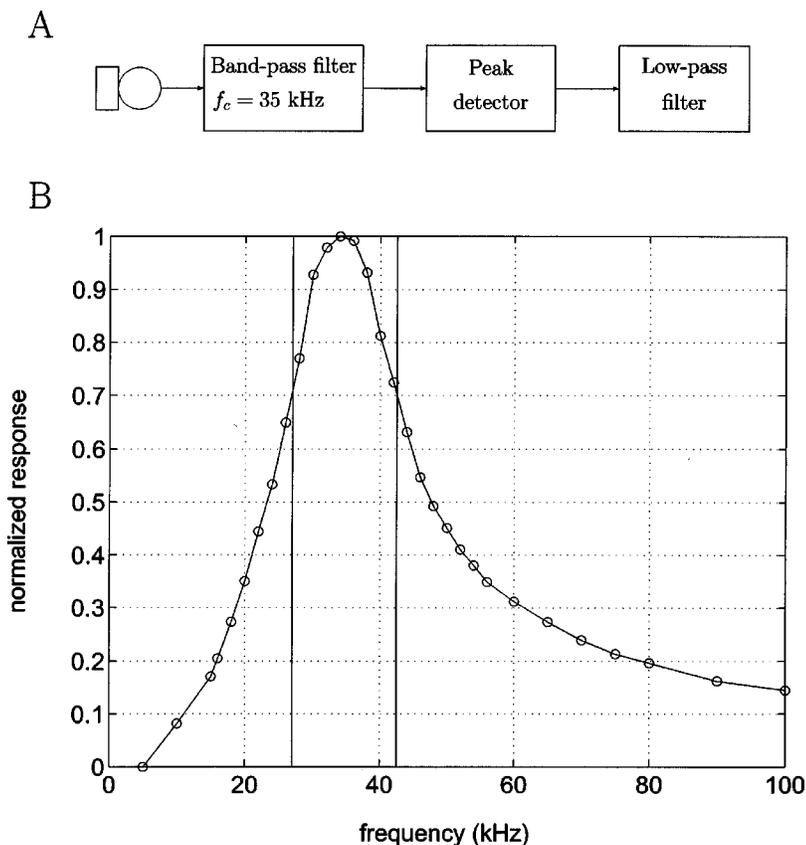
FIG. 3. (A) Schematic of signal-processing hardware. (B) Filter characteristics of the bandpass filter used. The  $x$  axis shows the frequency, while the  $y$  axis shows the normalized response. The vertical bars correspond to the 3-dB (half-power) points, i.e., the start and stop frequency. Examples of bandpass signal and envelope extraction may be seen in Figs. 4(A) and (B).
